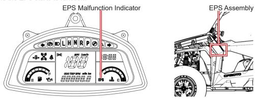
Each trouble code consists of 2 digits, denoted by the times of long flash and short flash of EPS MIL indicator. If there is a failure, the EPS indicator will start to flash. Do NOT switch off the machine. Check the flash sequence of EPS indicator. Write down the flash sequence and contact your dealer for diagnosis. Your dealer has the special tool required to diagnose, repair and clear trouble codes. Any codes will disappear once the problem has been diagnosed and repaired by your dealer.
